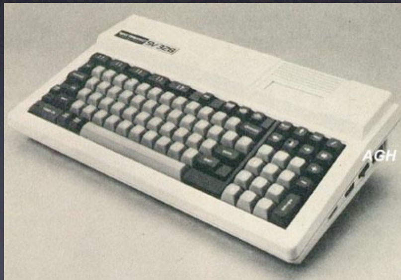
Spectravideo SV 328 (1983) Z80A / 3,6 MHz 64 KB RAM + 16 KB VRAM Full-stroke keyboard with numeric keypad Microsoft Extended Basic 40x24 Chars 16 colors / 256x192 pixel 3 channel sound 650 Euro
