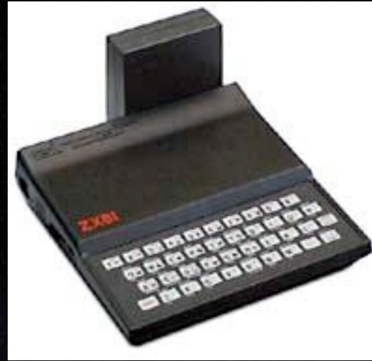
Sinclair ZX81 (1981) Z80A / 3,5 MHz 1 KB RAM + 16 KB expansion Basic QWERTY-keypad TV-output: 32x24 chars 64x44 block graphics 200 Euro
